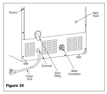
3. Remove 12 screws and back panel.
